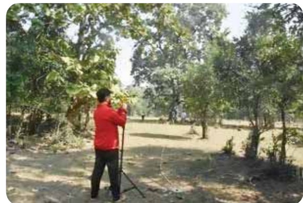
Measurement of tree diameter at different height segment Bastar forest division using Basal Area Finder (BAF)
