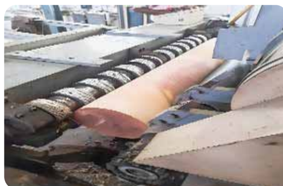
Coconut Trunk Veneering on Spindle less lathe
