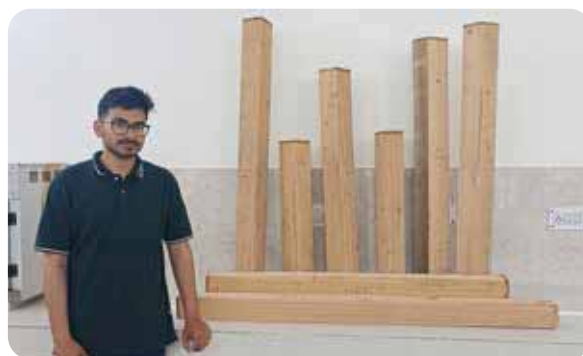
Building and construction grade (window and door frame/ railing main support/ handicrafts) sizes of Melia dubia dried in microwave vacuum dryer
