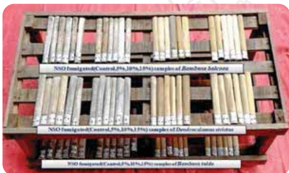
Field test of bamboo samples ( B. tulda , B. balcooa and D. strictus ) fumigated with different concentration of neem seed oil (Left) and pongamia seed oil (Right)
