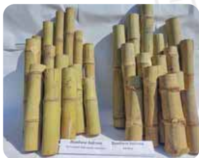
High intensity, Low intensity MW pre-treated bamboo drying quality
