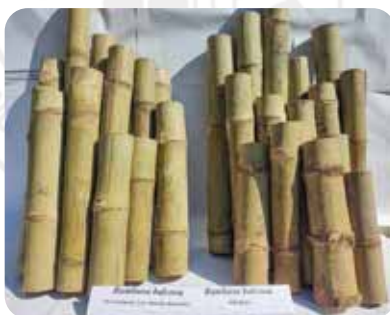
High intensity, Low intensity MW pre-treated bamboo drying quality
