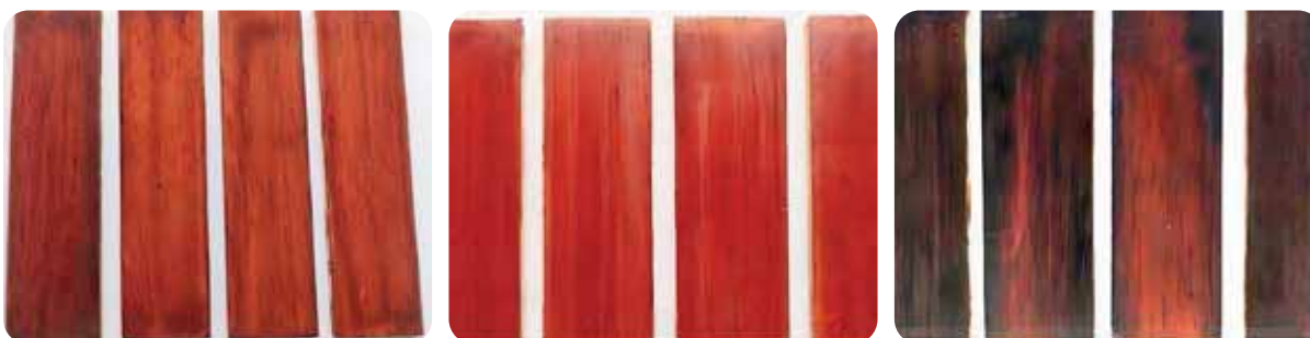
Rubber wood coated with Red Sanders bark extractive
