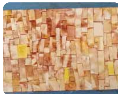
Preparation of oriented strand board from P. deltoides
