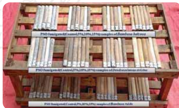
Field test of bamboo samples ( B. tulda , B. balcooa and D. strictus ) fumigated with different concentration of neem seed oil (Left) and pongamia seed oil (Right)
