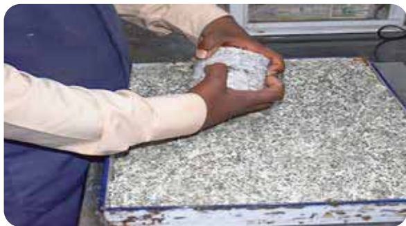
Particle board made by replacement of wood particles with currency briquettes particles
