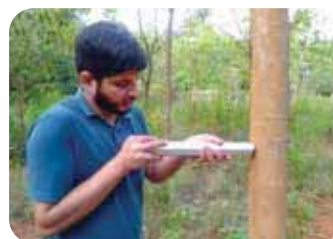
Recorded the penetration depth of Pylo-dyn pin in 15 selected trees at Nallal plantation, Karnataka
