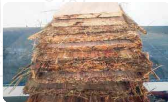
Preparation of destructured Bamboo Board from Bambusa balcooa
