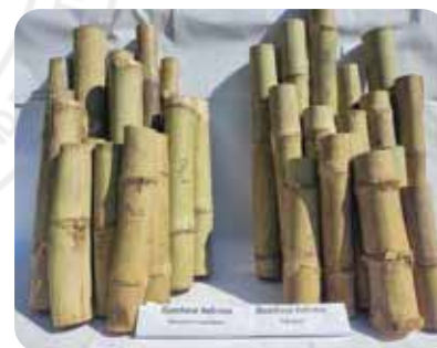
MWVD and conventional kiln dried B. balcooa
