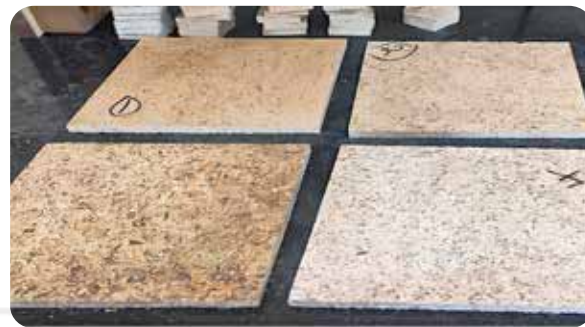
Particle board made by replacement of wood particles with currency briquettes particles
