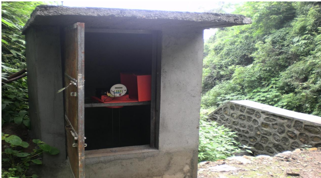
Automatic Digital Water Level Recorder Accuracy \pm 0.5 mm Battery operated
