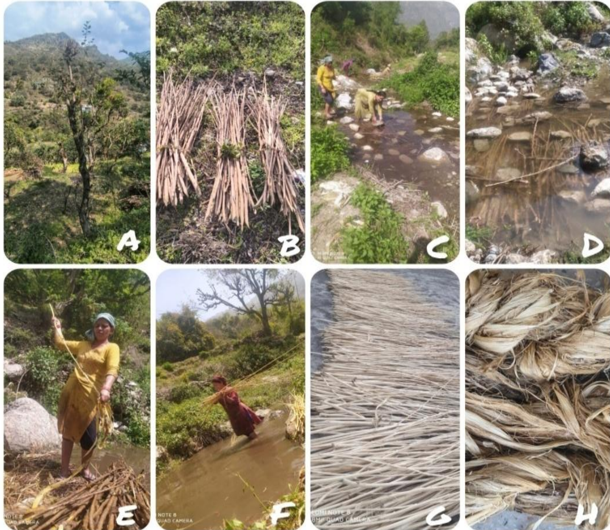
Fig.3: Retting process of Grewia optiva (A-Bhimal tree, B-Bundles of Bhimal branches, C-Preparing site for retting process, D-Bhimalbranches submerged in water for 30-40 days, E and F-Cleaning and separation of fibre,G and H-Extracted wood and fibre are sun dried)
