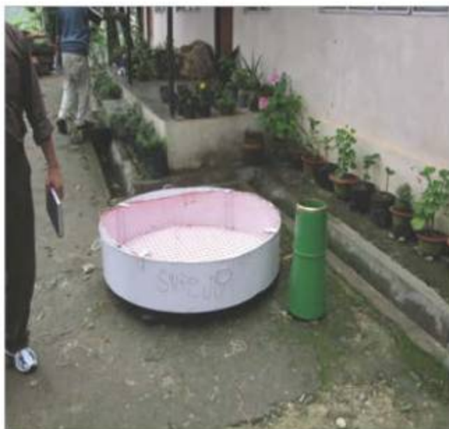
Figure 6.6: Rain-gauge, Evaporimeter and Double ring Infiltrometer installed at site, West Sikkim
