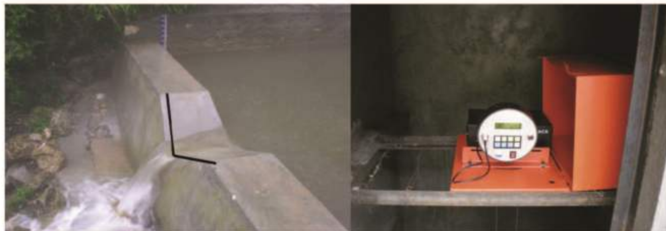
Figure 4.2: (a) V-notch sharp-crested weir (120° angles) with rectangular cross section and (b) Automatic Digital Water Level Recorder
