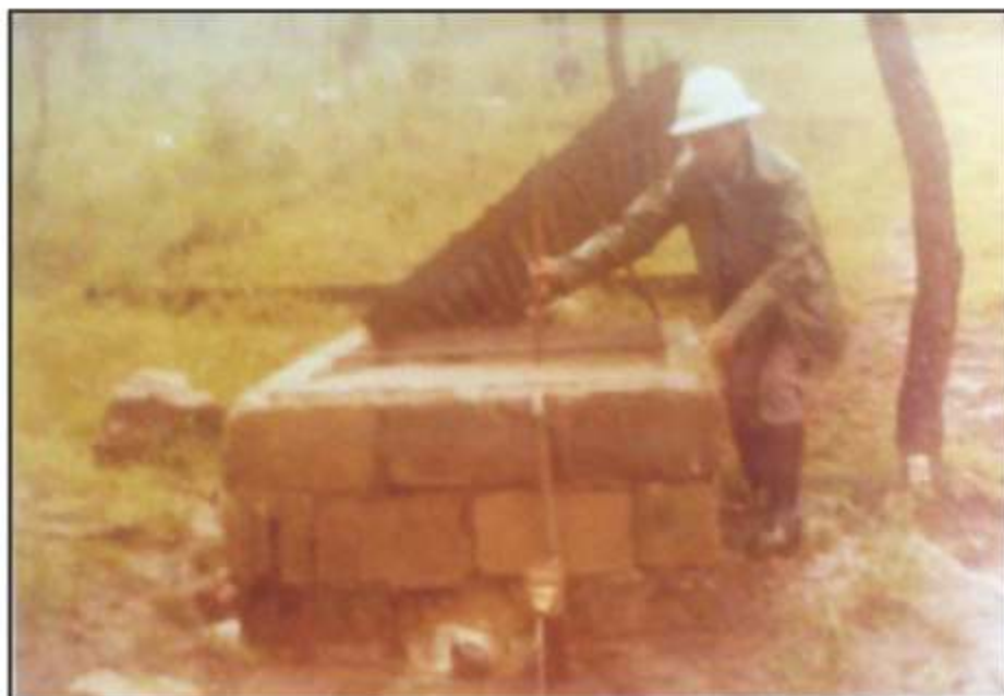
Figure 1.5: Water tight concrete trough constructed at the lower end of the plot for collecting surface runoff
