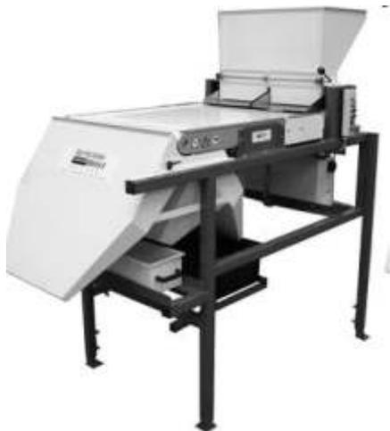
These machines use a magnetic force to separate damaged seeds or other particles from the good seeds.
