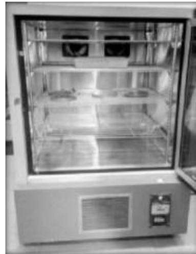
In plant incubator, heating, cooling and humidity are provided to reproduce certain environmental conditions for the growth and maintenance of plant. This is also used for germination studies in seed/plants.
