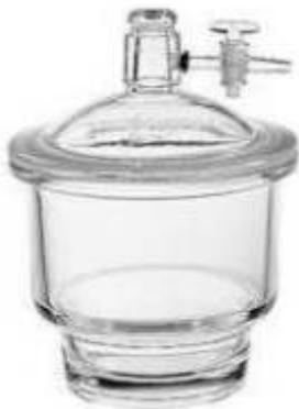
Desiccators protect seed from humidity and remove moisture from the seed samples. Desiccant like Silica gel or Calcium Chlorite are filled below the platform in the desiccators, which remove traces of water from the seed samples. The glass lid of the desiccator is sealed with grease or other lubricant to ensure an airtight seal.
