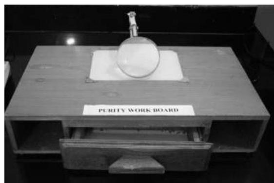
It is the instrument used for separating the inert matters from the seed samples. Inert matters can be anything other than the seeds like parts of leaves, stems, chaff, twigs, soil material, discolor and 1other foreign materials.
