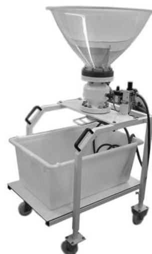
This seed density separation unit is used for accurate seed density grading using liquids (water or liquids with certain osmotic pressures). During separation the seeds should maintain the same moisture level content.
