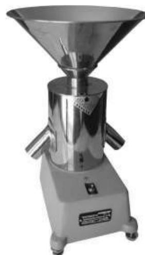
It is used for dividing and mixing of seed/grain which do accurate division and reduction to working size of samples exactly representative of the original sample.
