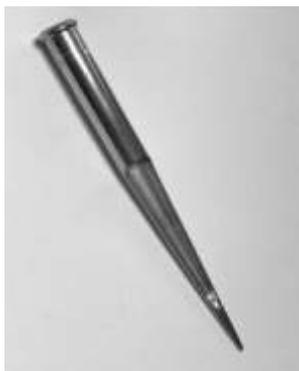
It is used for sampling seed from bag but not in bulk. It is inserted pointing upwards at an angle of about  $30^\circ$  to the horizontal, with the hole facing downwards until it reaches the centre of the bag, then revolved through  $180^\circ$ , bringing the hole face upwards, and is withdrawn with decreasing speed so that the quantity of seed obtained from successive locations increases progressively from centre to side of the bag.
