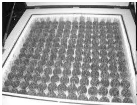
Thermogradient plates are set up in different ranges of temperature and this determines the exact temperature required for the germination of seeds. The gradient variation in temperature in sections is 0.5°C or 1°C.
